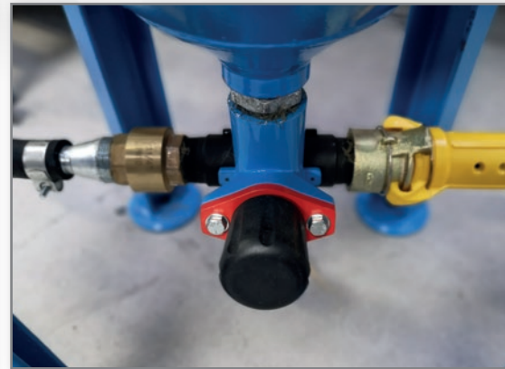
MICRO valve which dispenses the abradant.
